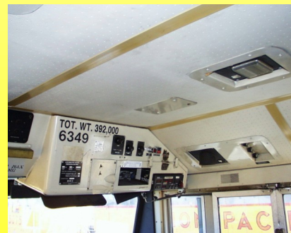
Locomotive Cab fitted with a New Vision Headliner Kit
